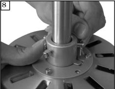
Install downrod into yoke. Align hole in downrod with hole in yoke and install cross pin. Install keeper into cross pin.
